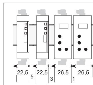
To allow the inserting of the  $\mu$ console: mount the instruments vertically (on horizontal DIN rail), leaving a 5 mm space between each.
