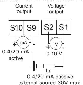
⚠ \* Only 1 of the 2 analog outputs can be activated at the same time (outputs not independent).
